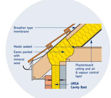
Figure 10 - Warm Pitched Roof - Gable/Verge Detail
