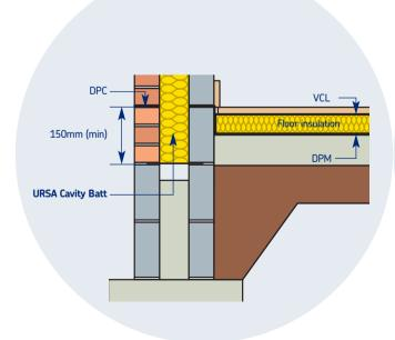
Figure 1 – Wall/Floor Junction
